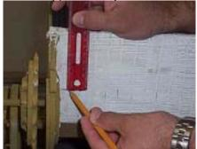
Step 8: Center the bar below the marked line. Scribe a line along the inside of the tab. Repeat on other side.
