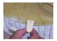
Step 3: Outline the Top Link Mount. Using a Track link, dry fit where the Top Link Mount fits snug against the Link. (Note - The backside of the link with the long tine should be facing up.) Mark the top link mount hole on the top of the turret.
